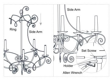
Screw out the set screw on the holder underside of the socket cap with Allen wrench. Insert the bottom end of the side arm into the holder. Secure by threading the set screws back in the holder. Hand tighten until snug.
