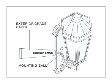
For assemble the MOUNTING BALLS, please note that you are required to apply a small amount of Silicone sealer to the threaded side of the MOUNTING BALLS and then install them onto the MOUNTING SCREWS.
